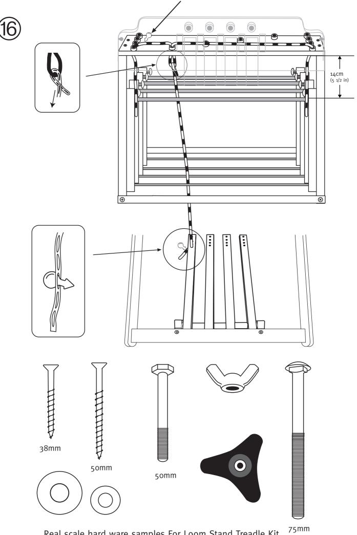
Real scale hard ware samples For Loom Stand Treadle Kit
